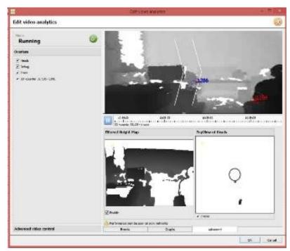
Check the overlay tick boxes to enable the overlays. These overlays provide debug information that enables the algorithm to be tuned, by altering the settings discussed in the section above, titled "Settings panel".
